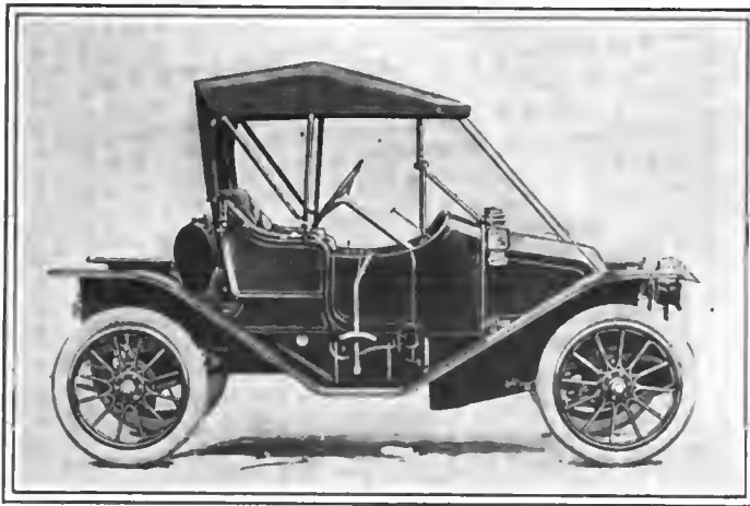
Fig. 5.—The Franklin fore-door roadster showing exterior position of speed-change lever
